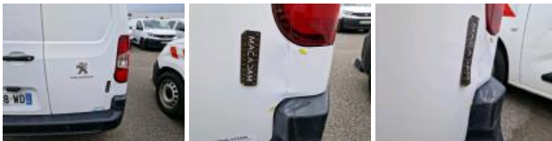
Rear light R, Broken, Replace
