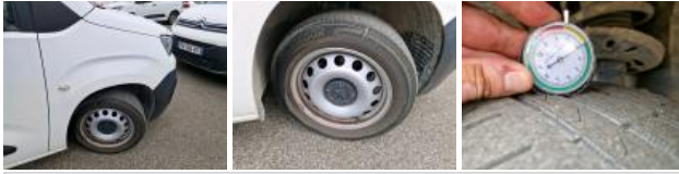
Tyre FL, Out of tolerance, Replace
