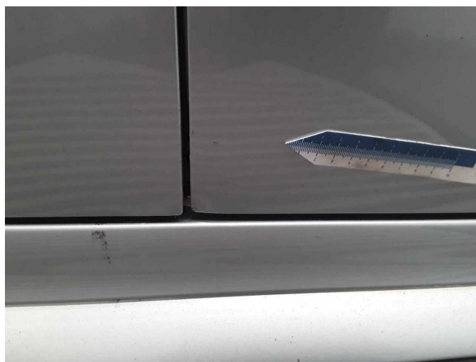
Damage 3: Door - front right side: Door - Deformed - Smooth repair work
