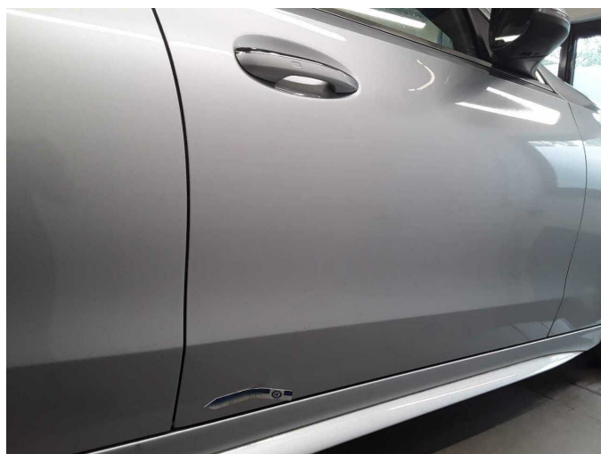
Damage 3: Door - front right side: Door - Deformed - Smooth repair work
