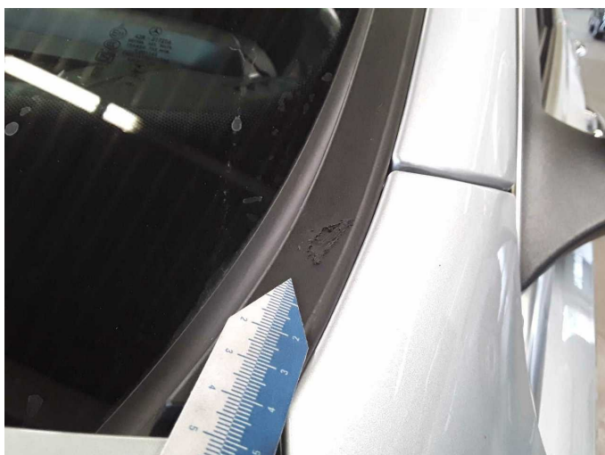
Damage 2: Vehicle glazing: Windscreen seal - Scratched - Replace
