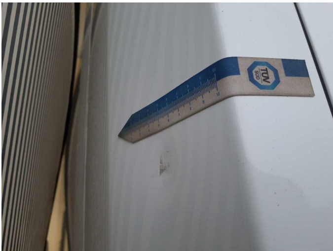
Damage 4: Side panel - rear left side: Side panel (Heckecke li.) - Dent / paintcoat damage - Smart repair
