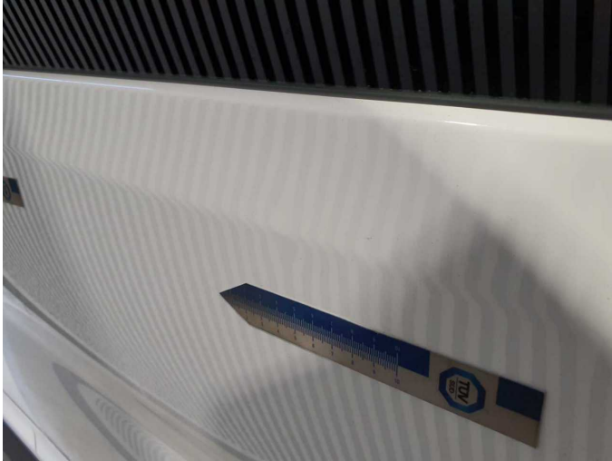
Damage 8: Sliding door, right: Sliding door - Deformed - Repair and paint
