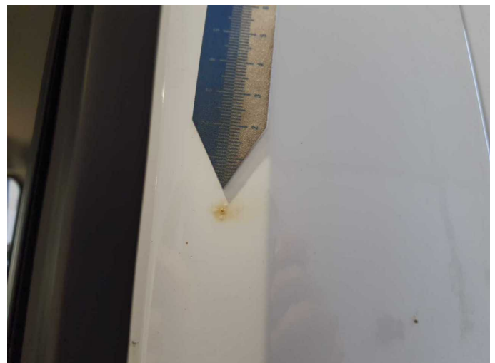
Damage 5: Door - front left side: Door - Corrosion - Smart repair
