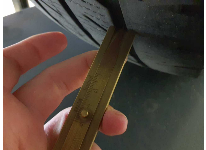
Damage 6: Wheel / tyres: Tyre - right - Does not meet the leasing specifications - Replace
