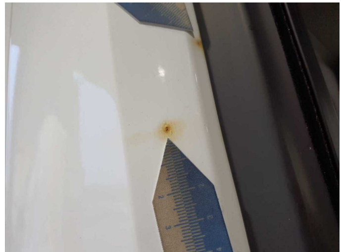
Damage 7: Door - front right side: Door - Corrosion - Repair and paint
