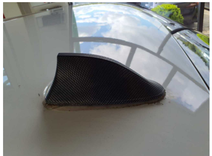
Damage 1: Roof: Aerial (Flosse statt Antenne mit Stab) - Differs from the original configuration
