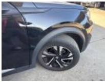
Tyre FL, Out of tolerance, Replace
