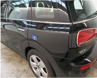
Wing Rear Left // Painting-scratch + dent
