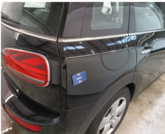
Wing Rear Right // Repair & Painting-scratch + dent
