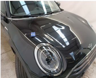
Front Bonnet // Repair & Painting-scratch + dent
