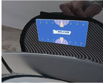
Wing Rear Left // Painting-scratch + dent
