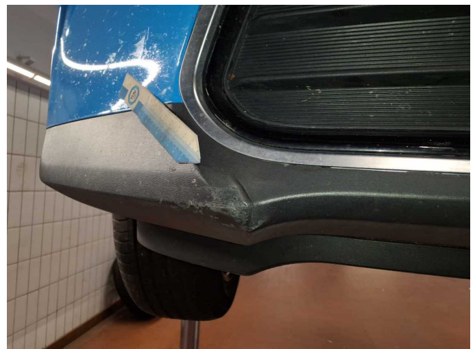
Damage 5: Front bumper: Spoiler (+ gestaucht) - Scratched - Replace
