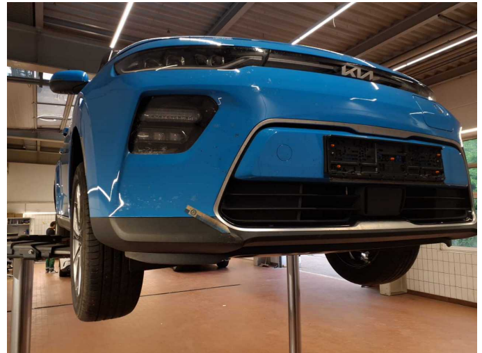
Damage 5: Front bumper: Spoiler (+ gestaucht) - Scratched - Replace
