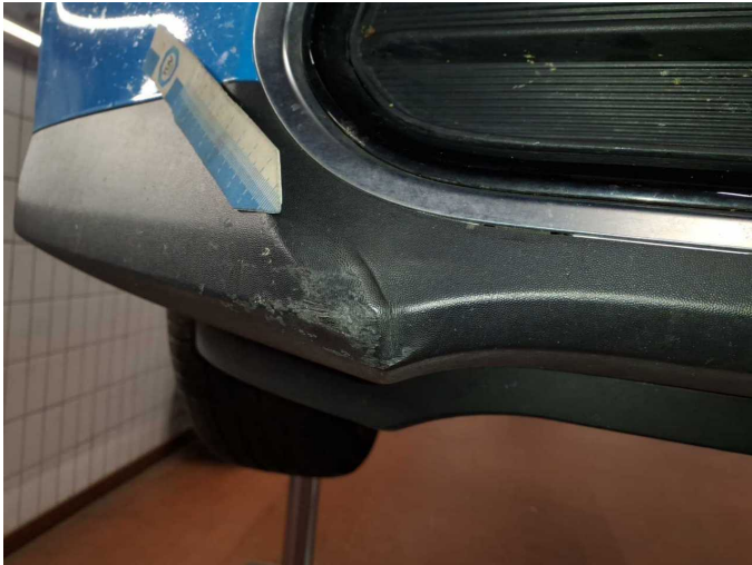
Damage 5: Front bumper: Spoiler (+ gestaucht) - Scratched - Replace
