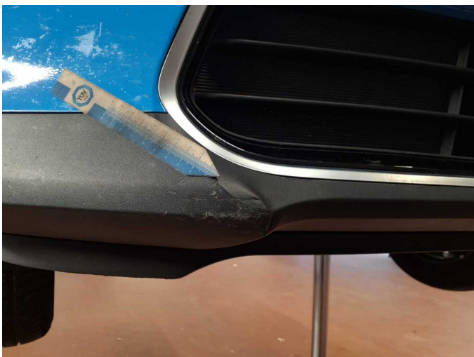
Damage 5: Front bumper: Spoiler (+ gestaucht) - Scratched - Replace
