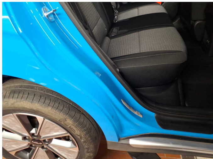
Wear and tear 1: Side panel - rear right side: Sill - dent(s) - No deduction
