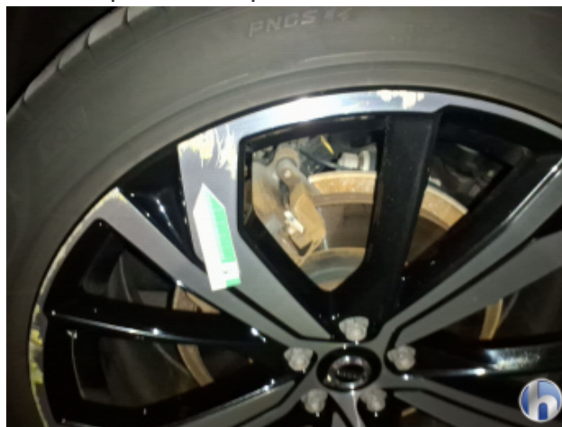
2. Felge Hinten - Links Kratzer - Smart Repair
