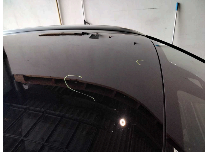
Damage 2: Roof: Roof - dent(s) - Smooth repair work
