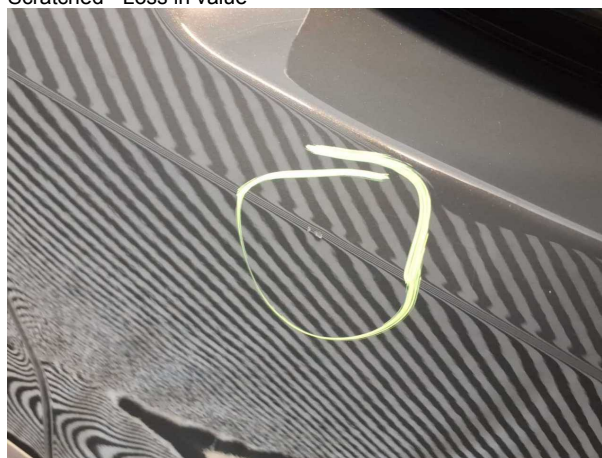
Damage #3: Door - front right side: Door - Dent / paintcoat damage - Smart repair
