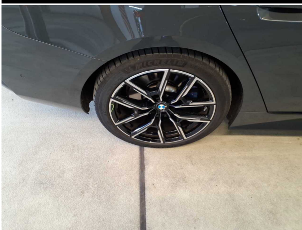
Damage #4: Wheel / tyres: Alloy rim - rear right side - Scratched - Loss in value
