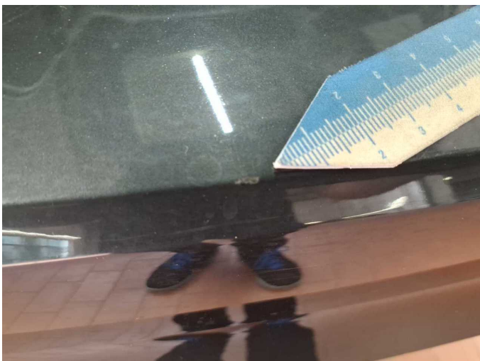
Damage 4: Rear bumper: Rear bumper - Scratched - Paint
