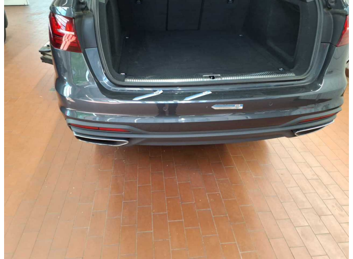
Damage 4: Rear bumper: Rear bumper - Scratched - Paint
