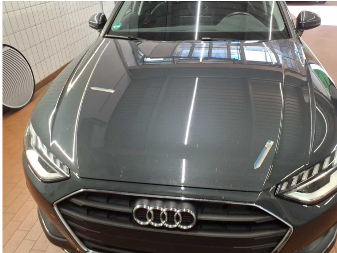
Damage 8: Bonnet: Bonnet - Stone chips - Paint
