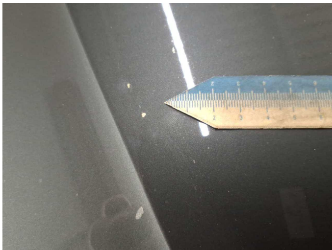
Damage 8: Bonnet: Bonnet - Stone chips - Paint
