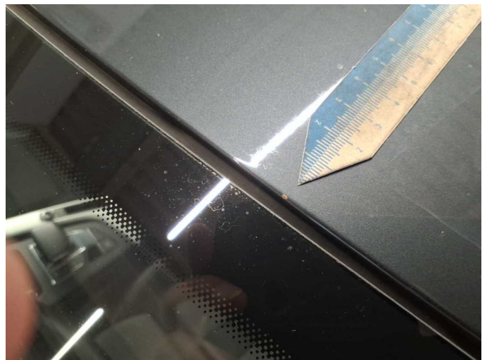
Damage 7: Roof: Roof (Steinschläge) - Corrosion - Paint
