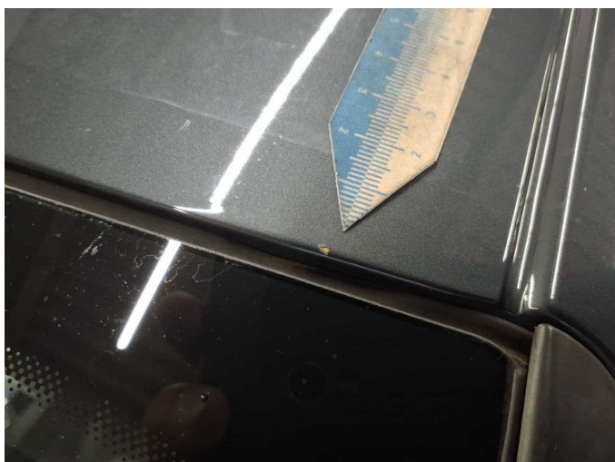
Damage 7: Roof: Roof (Steinschläge) - Corrosion - Paint
