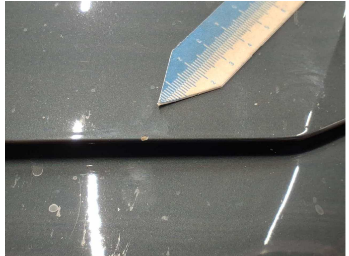
Damage 8: Bonnet: Bonnet - Stone chips - Paint
