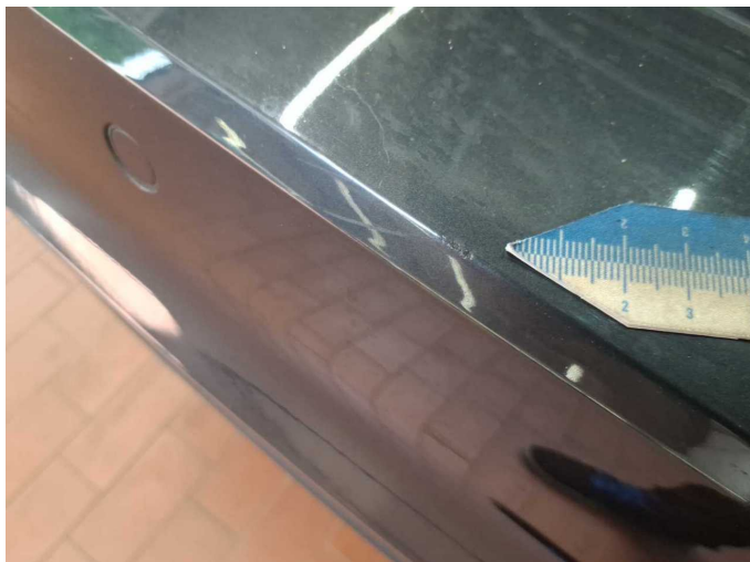
Damage 4: Rear bumper: Rear bumper - Scratched - Paint
