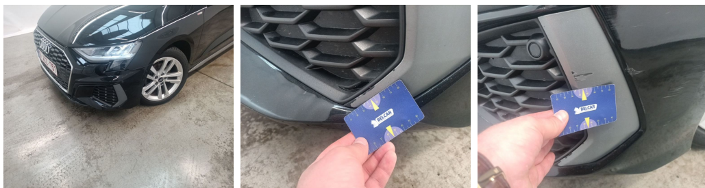
Bumper Front / Trim Left / Replace-scratch
