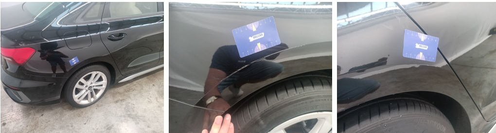
Wing Rear Right // Repair & Painting-scratch + dent
