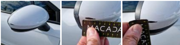
Outside rear-view mirror base R, Broken, Replace
