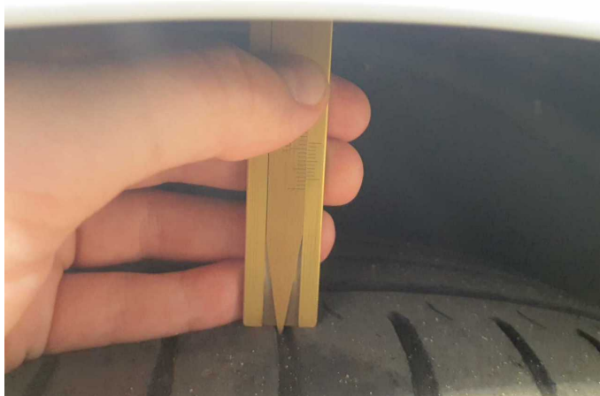
Damage 4: Wheel / tyres: Tyre - front - does not meet manufacturer specifications - Replace
