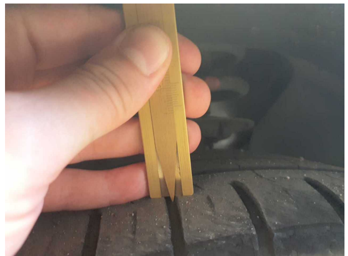
Damage 4: Wheel / tyres: Tyre - front - does not meet manufacturer specifications - Replace
