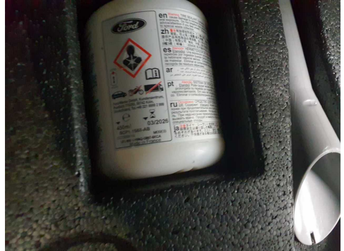
Damage 1: Equipment: Tirefit filler - Expired - Replace
