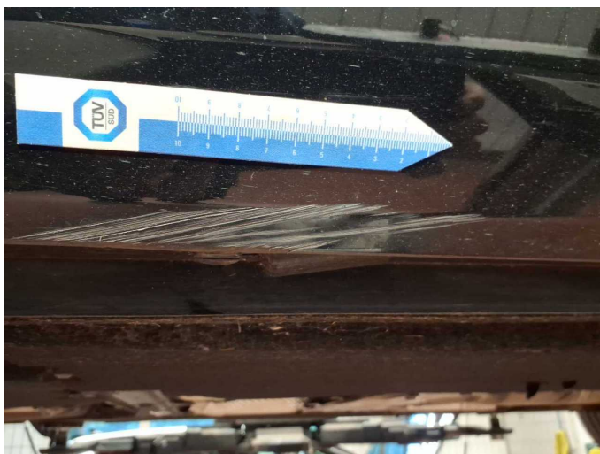
Damage 5: Sill - right side: Trim - Scratched - Paint
