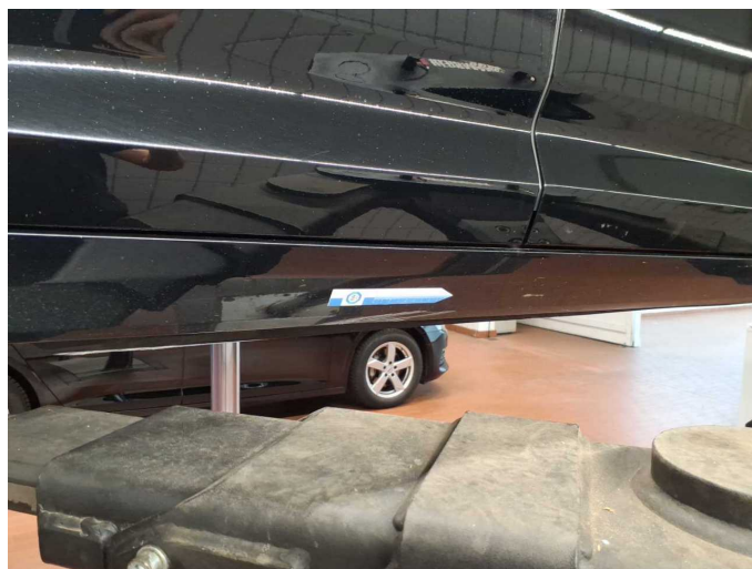
Damage 5: Sill - right side: Trim - Scratched - Paint
