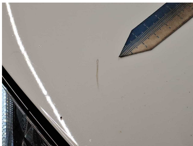
Damage 6: Bonnet: Bonnet - Dent / paintcoat damage - Paint
