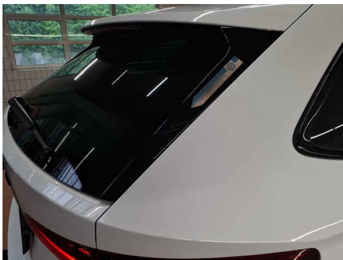
Damage 3: Trim / covers: Brightware / decorative strip (Heckklappe rechts) - Scratch(es) - Smart repair
