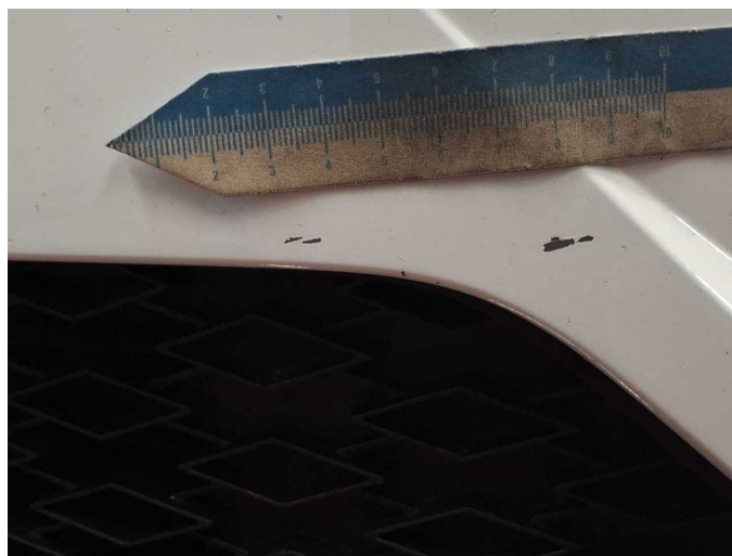
Damage 5: Front bumper: Front bumper - Scratch(es) - Paint
