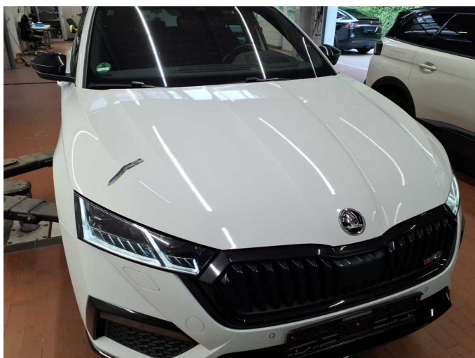
Damage 6: Bonnet: Bonnet - Dent / paintcoat damage - Paint
