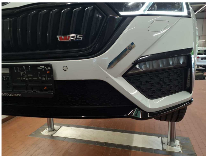
Damage 5: Front bumper: Front bumper - Scratch(es) - Paint
