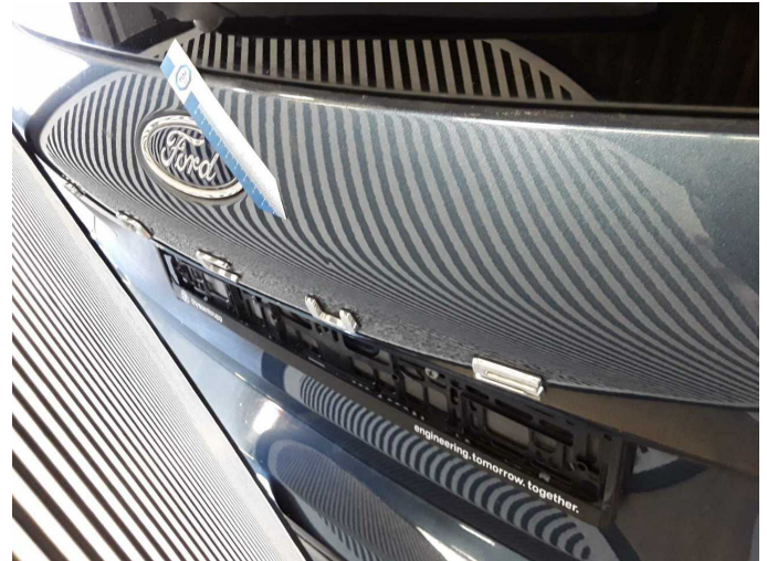
Wear and tear 2: Boot lid / rear door: Boot lid - dent(s) - Smooth repair work
