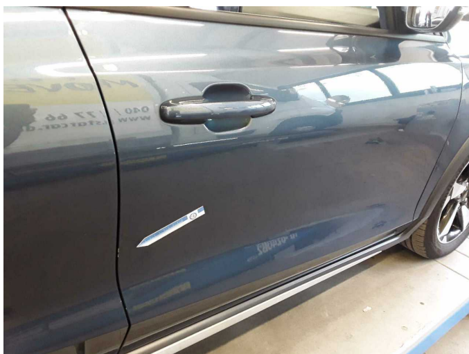
Wear and tear 4: Door - front right side: Door - Scratch(es) - Smart repair
