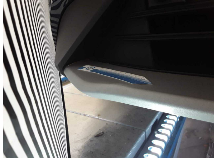
Damage 5: Front bumper: Spoiler (Blende) - Deformed - Replace
