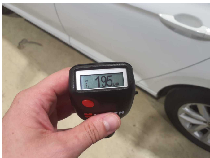
Repainting 4: Door - rear left side
