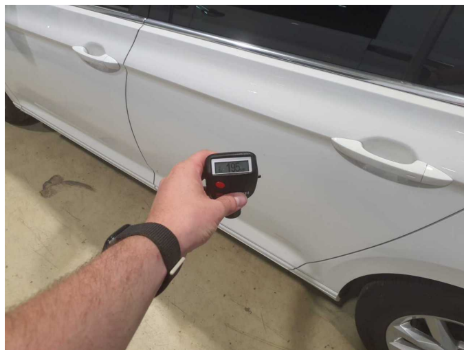
Repainting 4: Door - rear left side
