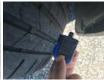
Tyre FL, Out of tolerance, Replace
