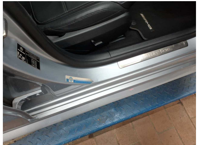
Damage 5: Sill - right side: Sill - dent(s) - Smooth repair work
