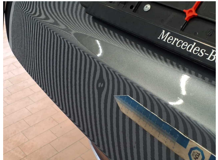
Damage 9: Boot lid / rear door: Boot lid (Ca. 8x) - dent(s) - Repair and paint
