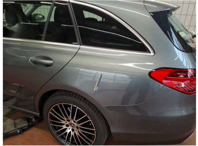
Damage 2: Side panel - rear left side: Side panel - Scratch(es) - Cover / polish
