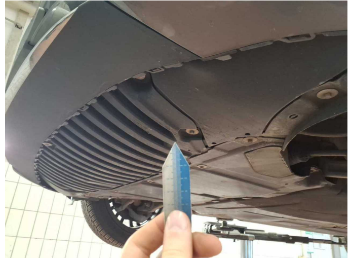
Wear and tear 1: Body: Underbody panelling - Scratched - No deduction
