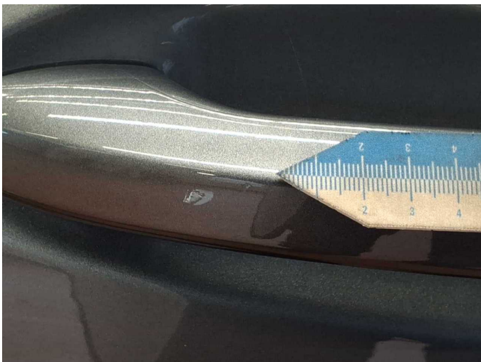
Damage 3: Door - rear left side: Door handle - outside - Scratch(es) - Smart repair
