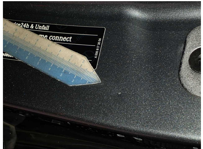
Damage 5: Body: B-pillar - left side - Dent / paintcoat damage - Smart repair
