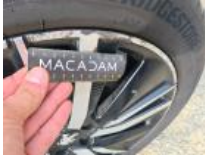
Tyre FR, Tear, Replace
