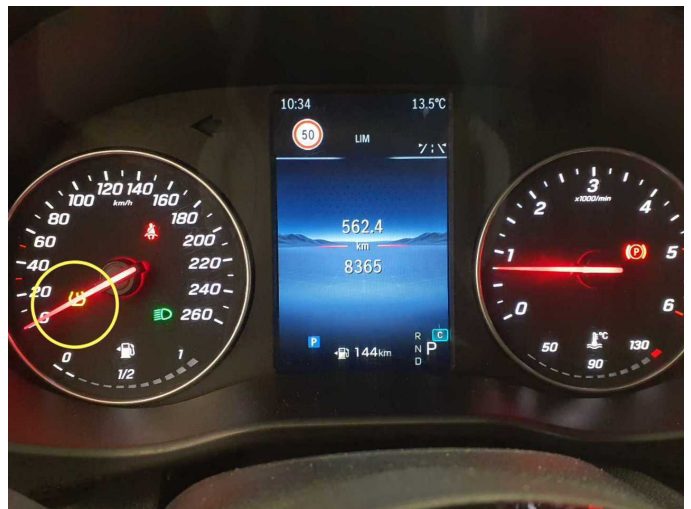
Damage 1: Instrument panel: Indicator light (Reifendruckkontrollsystem) - on - Perform diagnosis
