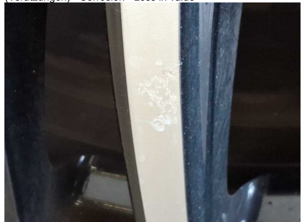
Damage #2: Wheel / tyres: Alloy rim - rear left side (Verätzungen) - Corrosion - Loss in value
