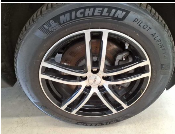
Damage #4: Wheel / tyres: Alloy rim - front right side - Corrosion - Loss in value
