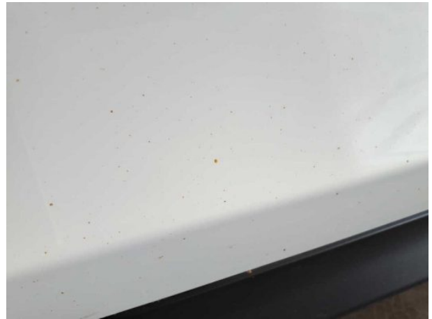
Damage #6: Body: Body (Flugrost) - Paint defect - Cover / polish
