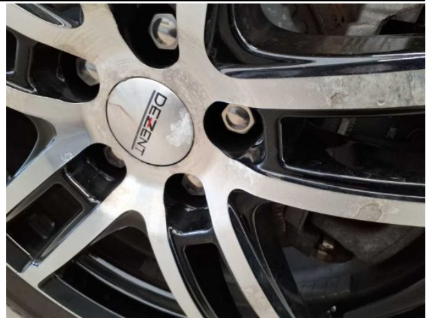
Damage #4: Wheel / tyres: Alloy rim - front right side - Corrosion - Loss in value
