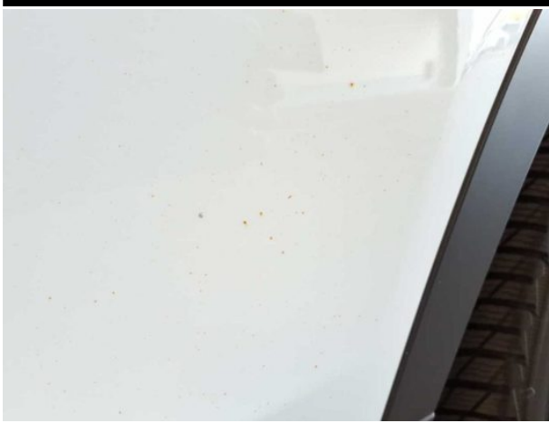
Damage #6: Body: Body (Flugrost) - Paint defect - Cover / polish
