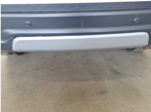
Damage #5: Rear bumper: Spoiler - Deformed - Replace
