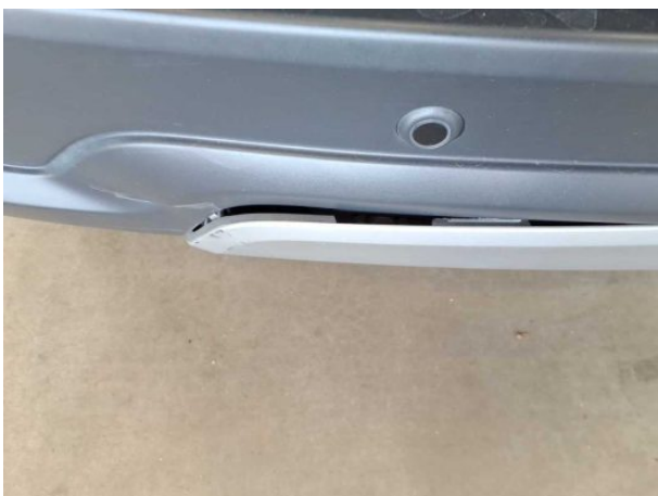
Damage #5: Rear bumper: Spoiler - Deformed - Replace
