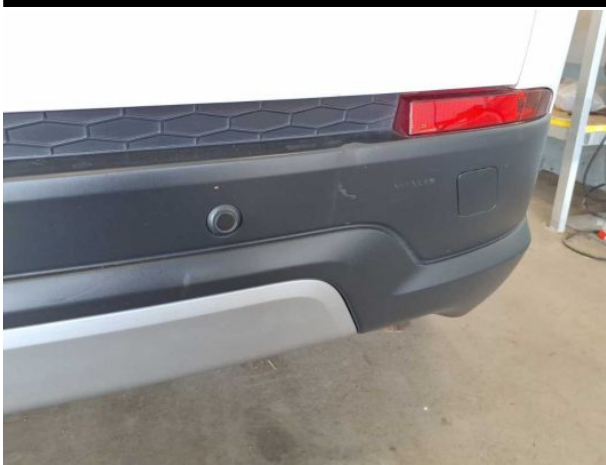
Damage #7: Rear bumper: Rear bumper (unpainted) - Deformed - Replace
