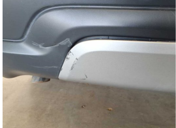
Damage #5: Rear bumper: Spoiler - Deformed - Replace
