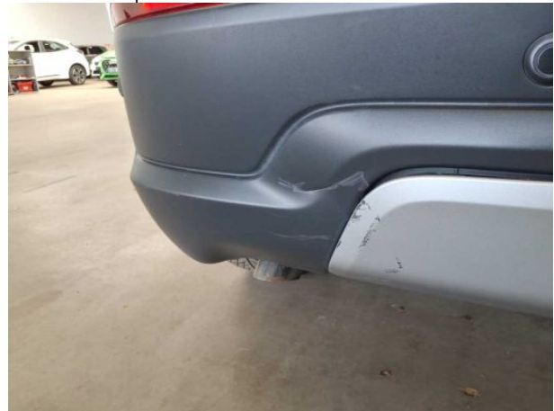
Damage #7: Rear bumper: Rear bumper (unpainted) - Deformed - Replace
