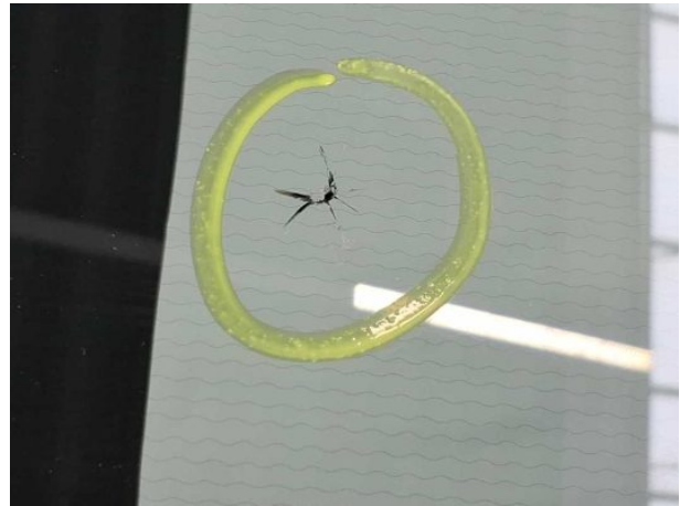
Damage #8: Vehicle glazing: Windscreen with lane departure assistant - Stone chips - Replace
