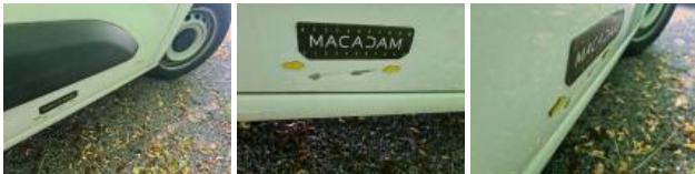
Sliding door R, Dent(s) and scratch(es), Repair and paint (complete)
