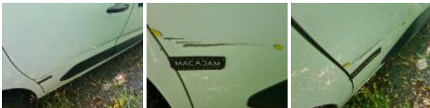
Bumper corner RL, Hole, Replace
