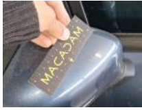
Outside rear-view mirror housing R, Scratch(es), Acceptable
