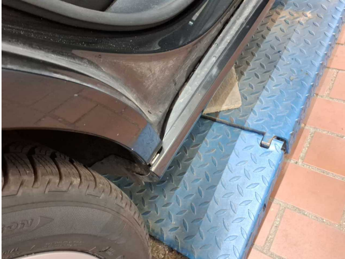
Damage 2: Sill - right side: Trim - Loose - Repair
