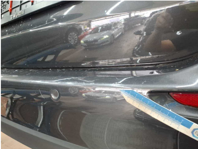
Damage 7: Rear bumper: Rear bumper - Scratch(es) - Paint
