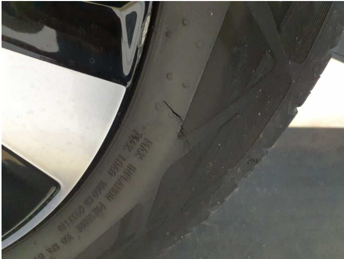
Damage 20: Wheel / tyres: Tyre - front left side (nicht fahrbereit) - Broken / torn - Replace
