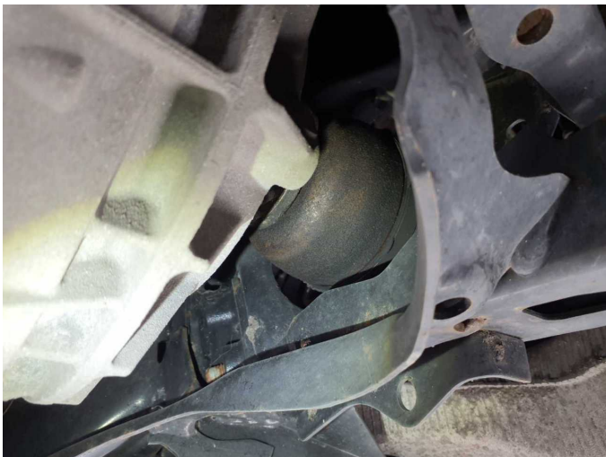
Damage 2: Rear axle: Differential - Leaking - Perform diagnosis
