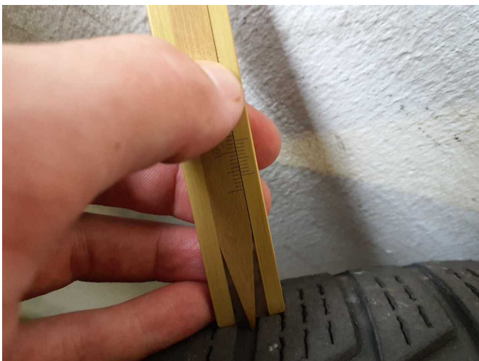
Wear and tear 7: 2nd wheel set: 2 tyres - does not meet manufacturer specifications - No deduction
