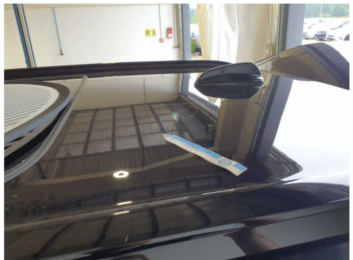
Wear and tear 9: Roof: Roof - dent(s) - Smooth repair work
