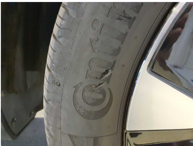
Damage 21: Wheel / tyres: Tyre - front right side (nicht fahrbereit) - Broken / torn - Replace
