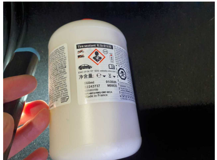
Damage 3: Equipment: Tirefit filler - Expired - Replace
