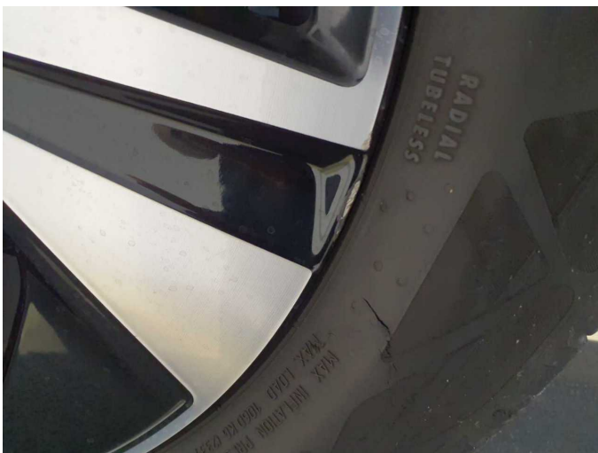
Damage 19: Wheel / tyres: Alloy rim - front left side - Scratch(es) - Loss in value
