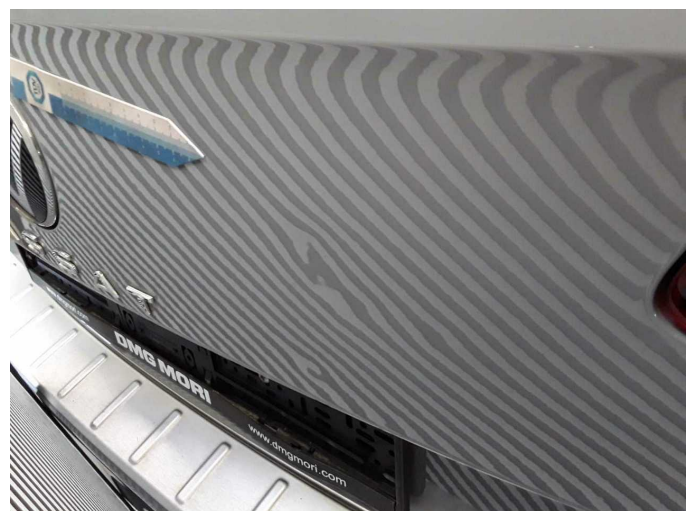
Damage 4: Boot lid / rear door: Boot lid - Deformed - Smart repair
