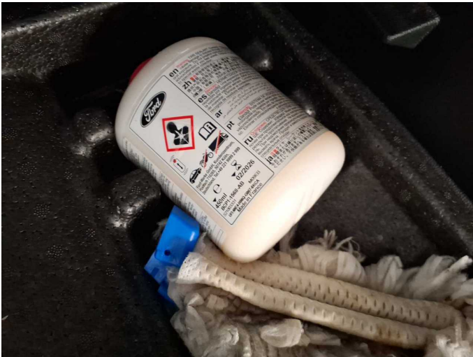
Damage 1: Equipment: Tirefit filler - Expired - Replace
