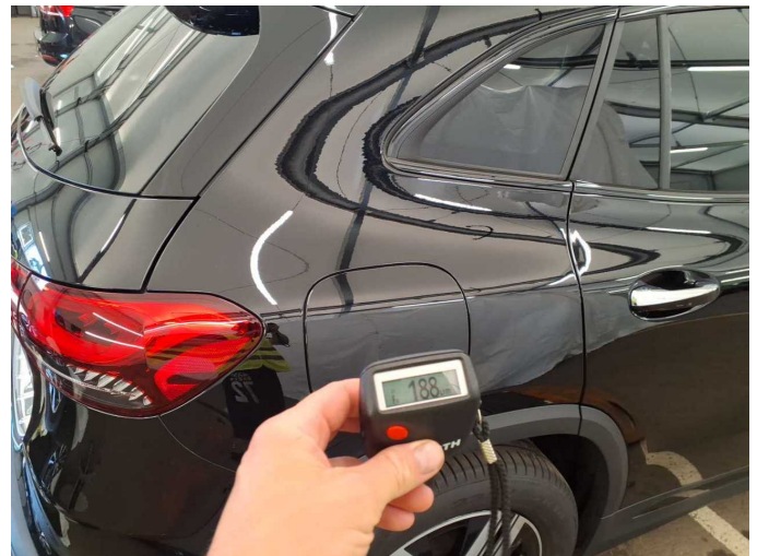
Repainting 1: Side panel - rear right side
