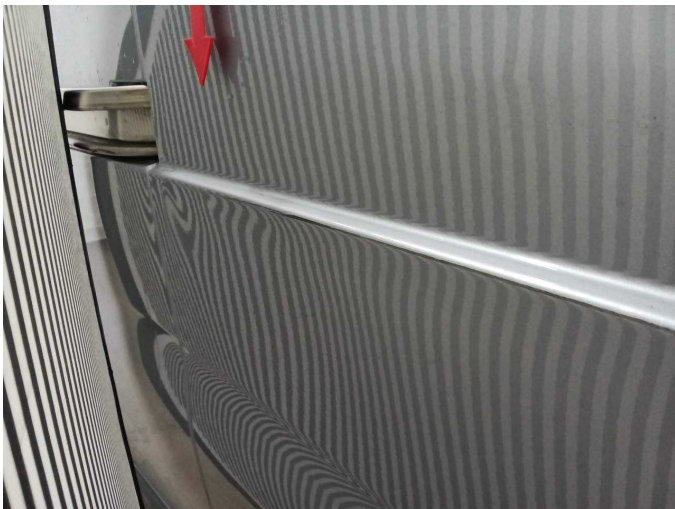
Damage 13: Sliding door, right: Sliding door - Dent / paintcoat damage - Repair and paint
