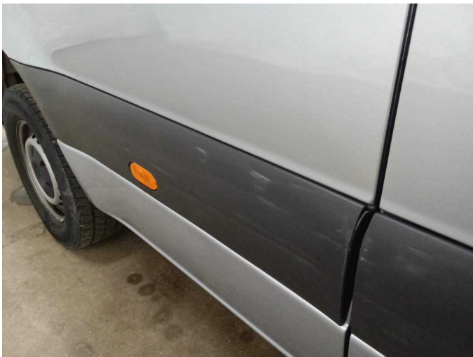
Damage 5: Side panel - rear right side: Protection strip - Broken / torn - Replace
