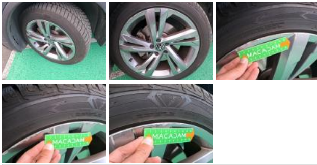
Tyre RL, Out of tolerance, Replace
