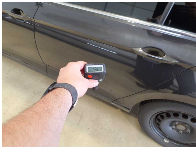
Repainting 2: Door - rear left side
