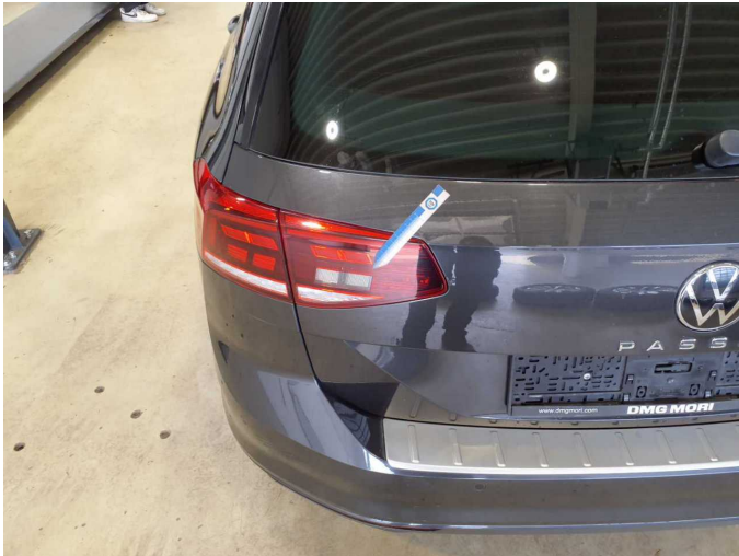
Damage 8: Tail light: Tail lamp - left side - Broken / torn - Replace
