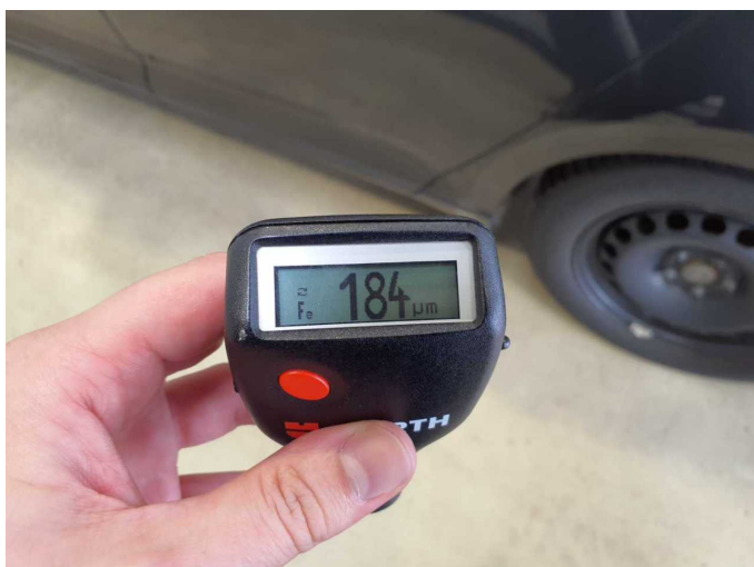
Repainting 2: Door - rear left side
