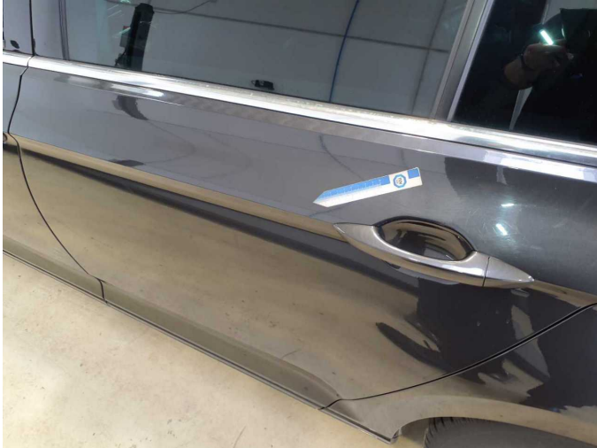
Damage 11: Door - rear left side: Door - Scratch(es) - Paint
