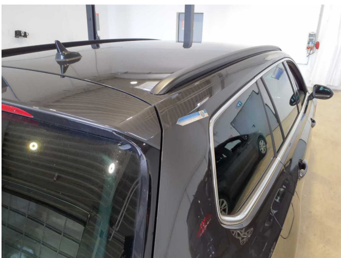
Damage 10: Roof: Roof rail - right side (Anätzung) - Paint defect - Repair and paint
