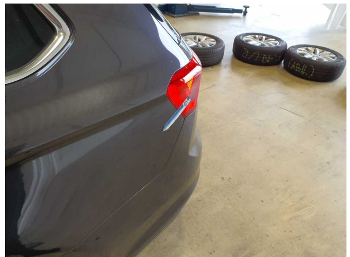
Damage 4: Side panel - rear left side: Side panel - Dent / paintcoat damage - Smart repair
