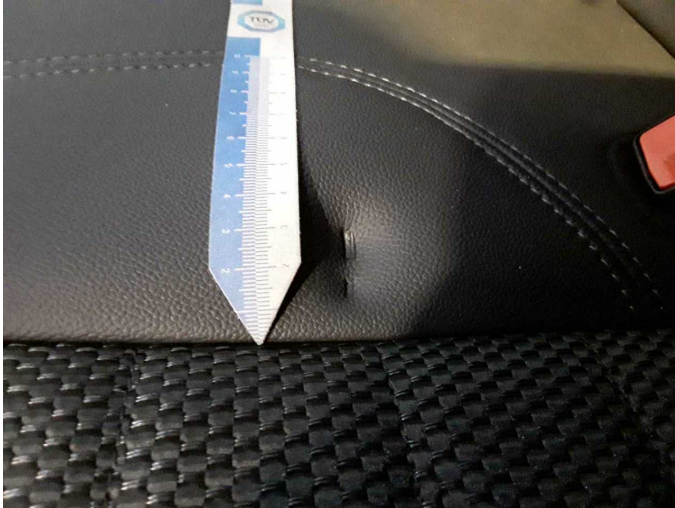
Damage 2: Seat - rear: Upholstery (Abdruck) - Deformed - Loss in value
