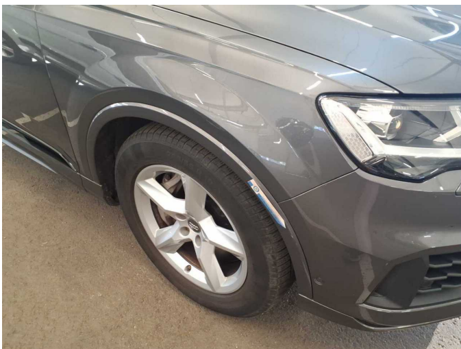
Damage 6: Mudguard - right side: Wheel well extension - Scratched - Replace
