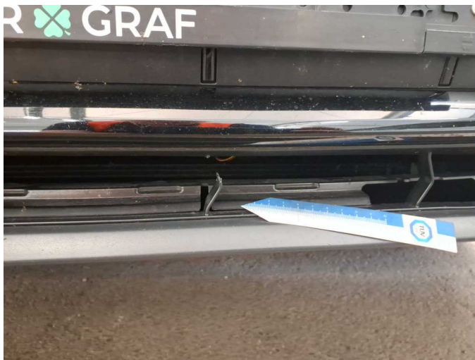
Damage 8: Front bumper: Air-inlet grille - Broken / torn - Replace
