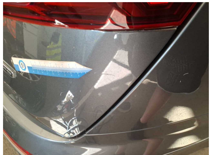
Damage 7: Boot lid / rear door: Boot lid - Dent / paintcoat damage - Repair and paint
