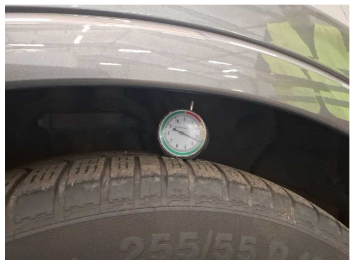
Damage 9: Wheel / tyres: Tyres - complete set (4x 3mm) - Does not meet the leasing specifications - Replace
