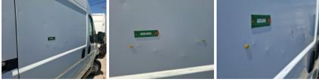
Central pillar R, Dent(s), Repair and paint (complete)
