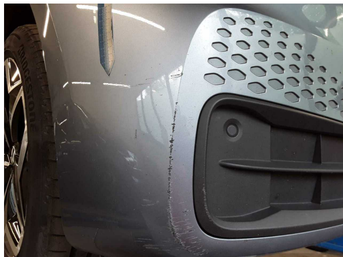
Damage 9: Front bumper: Front bumper - Scratched - Paint
