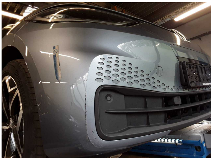
Damage 9: Front bumper: Front bumper - Scratched - Paint
