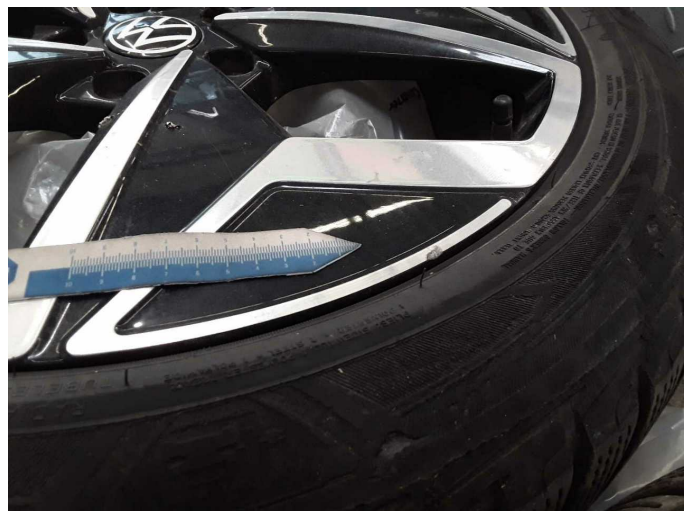
Damage 4: 2nd wheel set: 2 alloy rims - Scratch(es) - Loss in value
