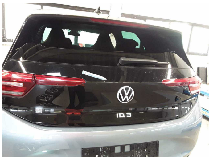
Damage 10: Boot lid / rear door: Boot lid - Scratched - Paint
