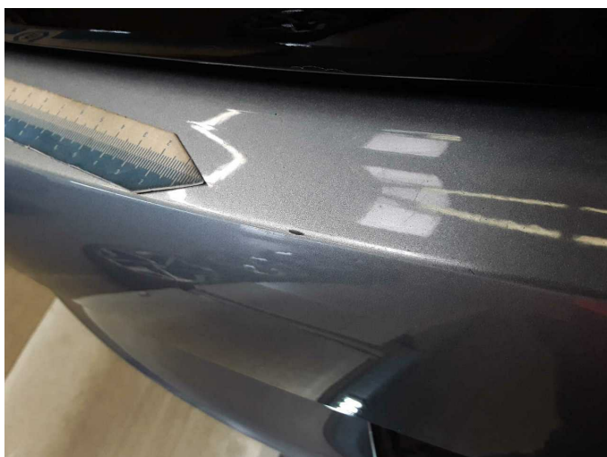
Damage 8: Rear bumper: Rear bumper - Scratch(es) - Paint
