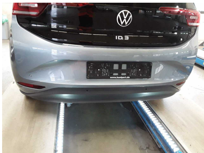
Damage 8: Rear bumper: Rear bumper - Scratch(es) - Paint
