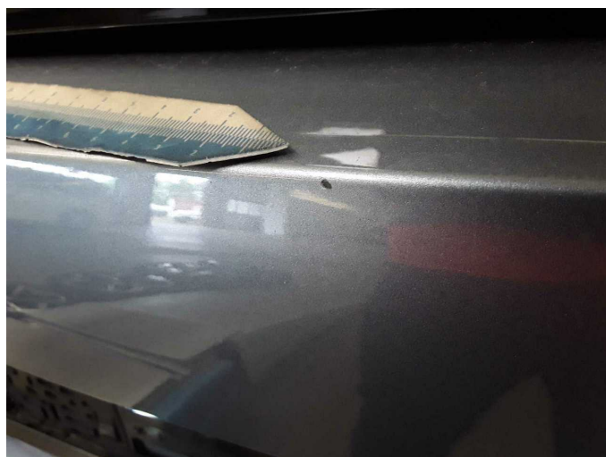
Damage 8: Rear bumper: Rear bumper - Scratch(es) - Paint
