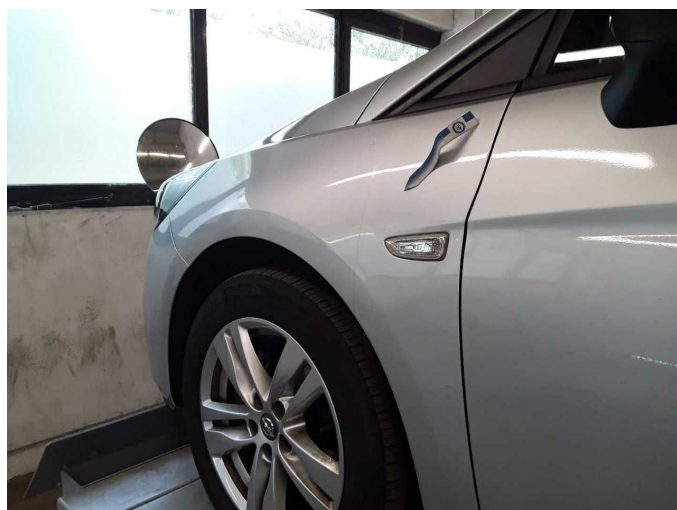
Damage 9: Mudguard - left side: Mudguard - left side - Deformed - Replace
