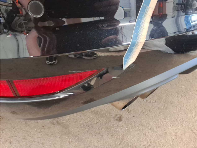
Damage 5: Rear bumper: Rear bumper - Scratch(es) - Paint
