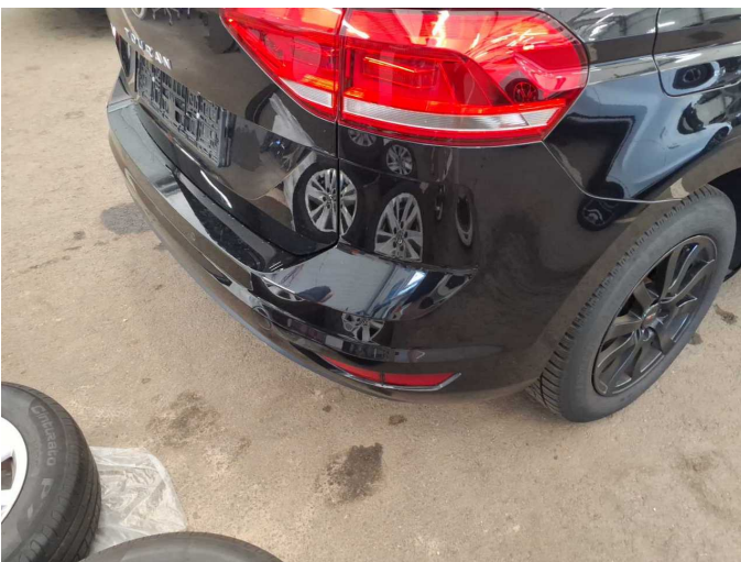
Damage 5: Rear bumper: Rear bumper - Scratch(es) - Paint
