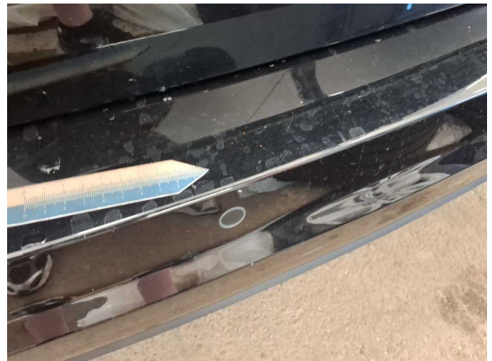
Damage 5: Rear bumper: Rear bumper - Scratch(es) - Paint
