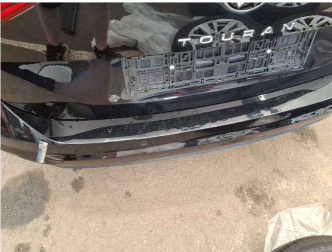
Damage 5: Rear bumper: Rear bumper - Scratch(es) - Paint
