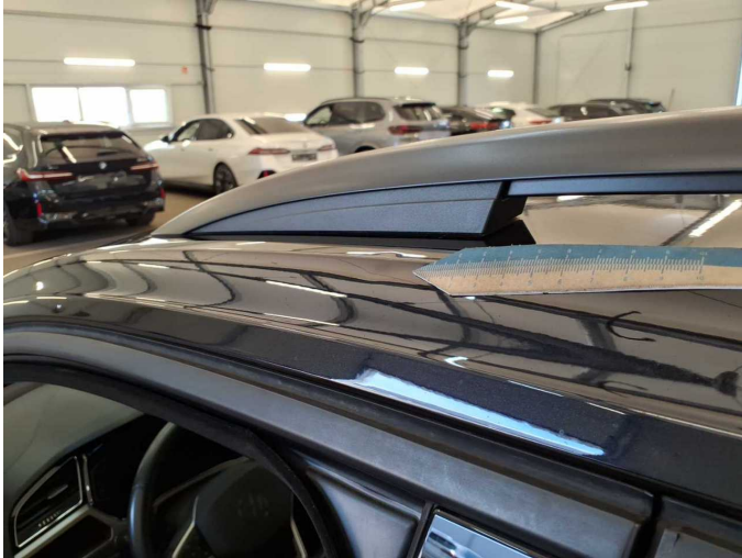
Damage 1: Roof: Roof rail - left side - dent(s) - Smooth repair work
