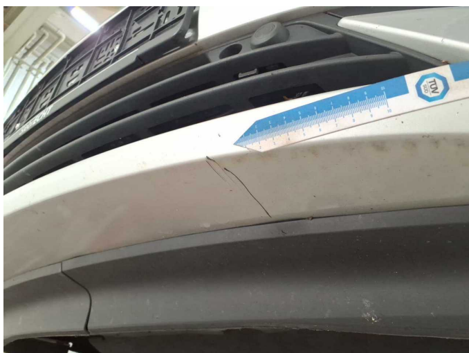
Damage 1: Front bumper: Spoiler - Scratch(es) - Smart repair
