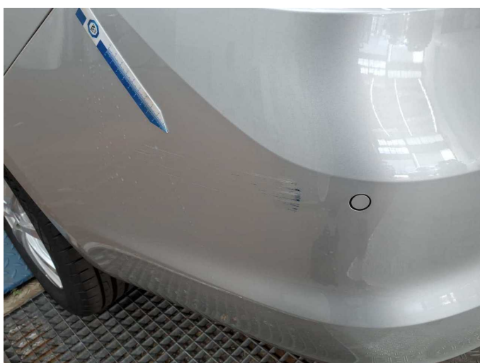
Damage 2: Rear bumper: Rear bumper - Scratch(es) - Paint
