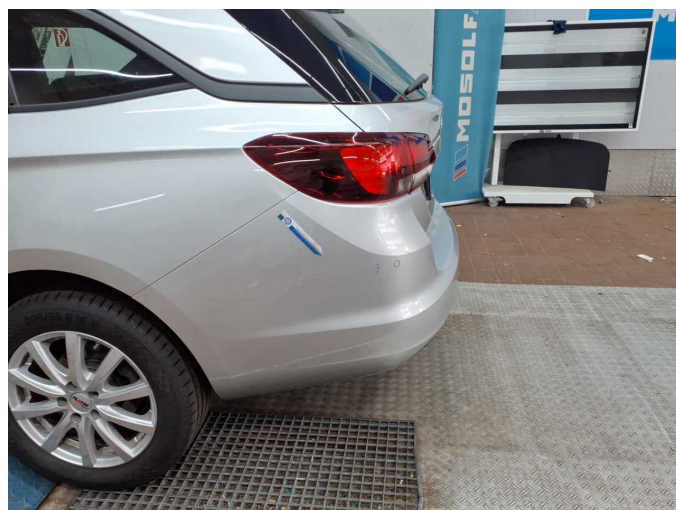
Damage 2: Rear bumper: Rear bumper - Scratch(es) - Paint
