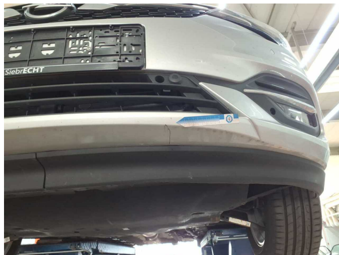
Damage 1: Front bumper: Spoiler - Scratch(es) - Smart repair
