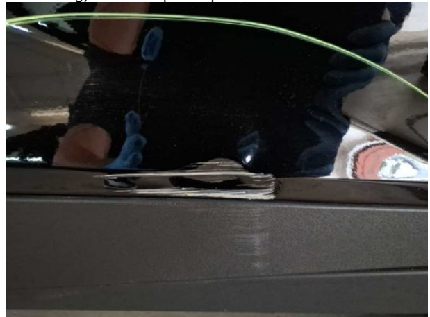
Damage #18: Door - rear left side: Door - Damaged - Replace
