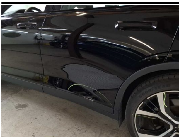
Damage #14: Door - rear left side: Brightware - lower - Scratched - Replace
