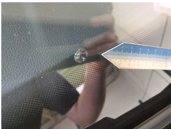
Damage 15: Vehicle glazing: Windscreen - Stone chips - Replace
