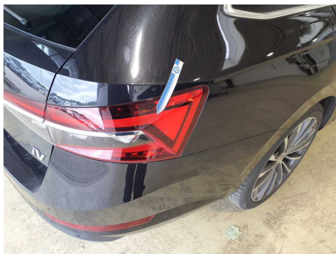
Damage 6: Tail light: Tail lamp - right side - Broken / torn - Replace
