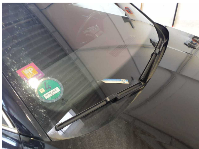
Damage 15: Vehicle glazing: Windscreen - Stone chips - Replace
