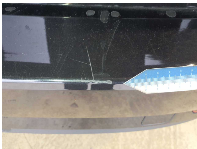
Damage 8: Rear bumper: Rear bumper - Scratch(es) - Paint
