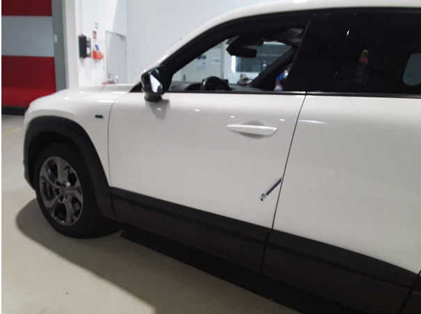
Beschädigung #1: Tür vorn links: Tür - Kratzer - Smart Repair
