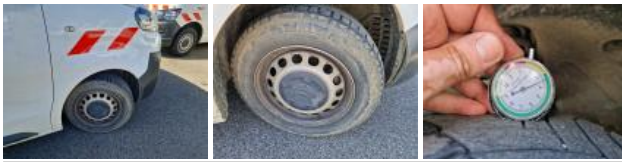
Tyre FL, Out of tolerance, Replace
