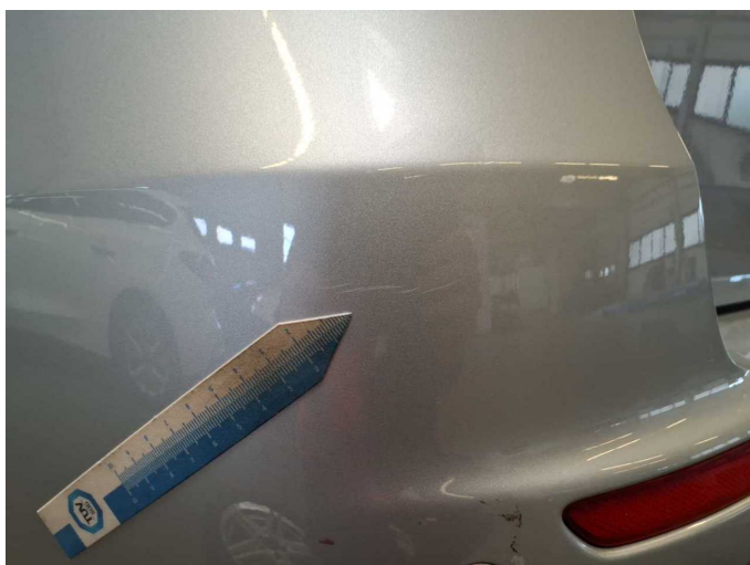
Damage 9: Rear bumper: Rear bumper - Scratch(es) - Paint
