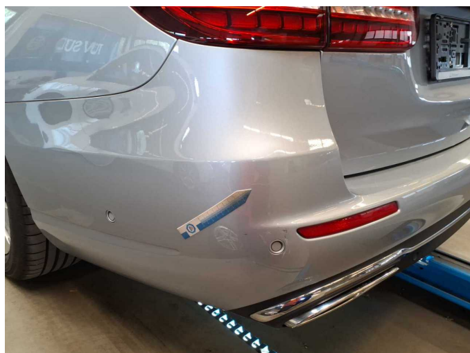
Damage 9: Rear bumper: Rear bumper - Scratch(es) - Paint
