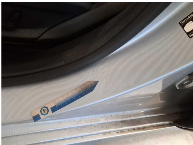
Damage 7: Sill - left side: Sill - dent(s) - Smooth repair work
