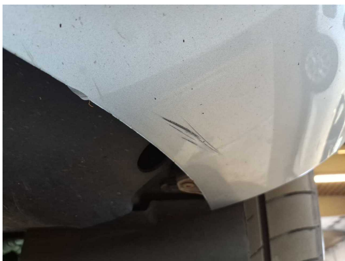
Damage 8: Front bumper: Front bumper (+ Steinschläge) - Scratch(es) - Paint
