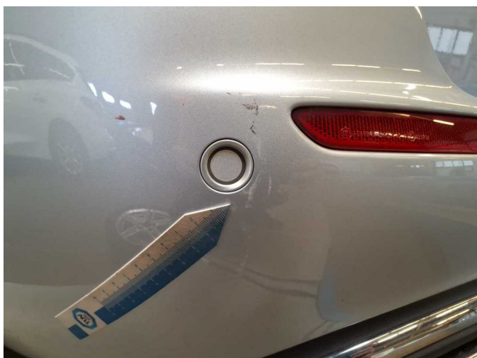
Damage 9: Rear bumper: Rear bumper - Scratch(es) - Paint
