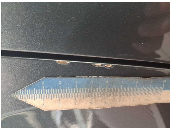
Damage 17: Side panel - rear right side: Side panel - Scratch(es) - Paint
