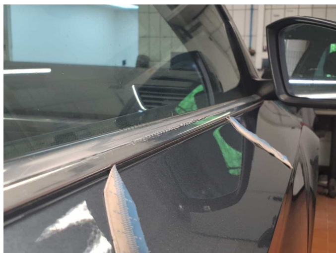
Damage 7: Door - front right side: Strip - outer - Scratch(es) - Replace
