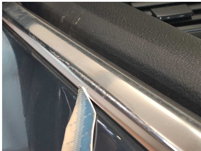
Damage 6: Door - front left side: Strip - outer - Scratch(es) - Replace
