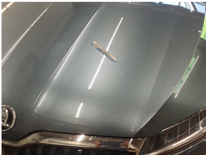
Damage 20: Bonnet: Bonnet (+ Steinschläge) - Paint defect - Paint
