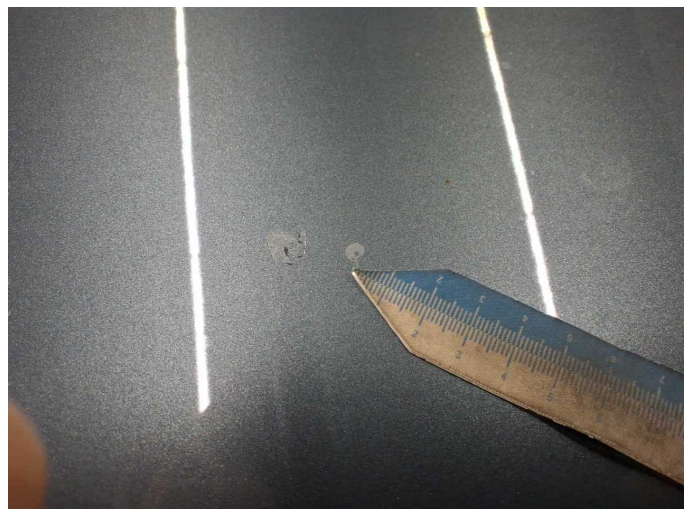
Damage 20: Bonnet: Bonnet (+ Steinschläge) - Paint defect - Paint
