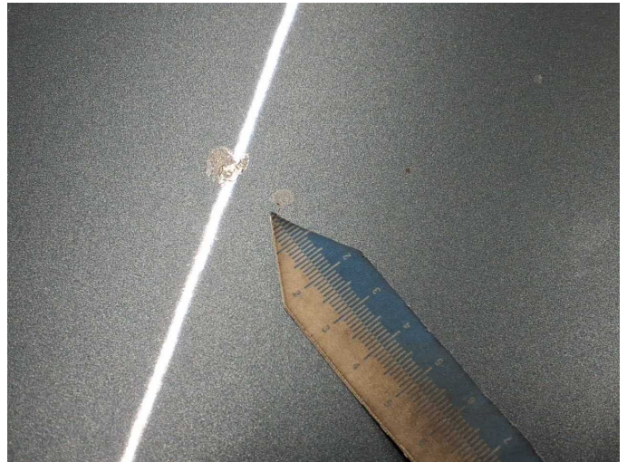
Damage 20: Bonnet: Bonnet (+ Steinschläge) - Paint defect - Paint
