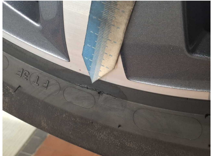
Damage 14: Wheel / tyres: Tyre - front right side (nicht fahrbereit) - Broken / torn - Replace
