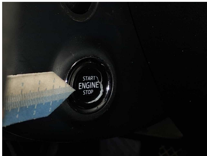
Damage 8: Steering system: Steering column (Taster Startknopf) - Broken / torn - Loss in value
