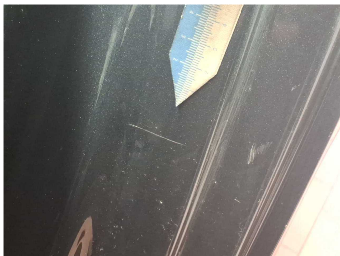
Damage 12: Side panel - rear left side: Sill - Scratch(es) - Smart repair
