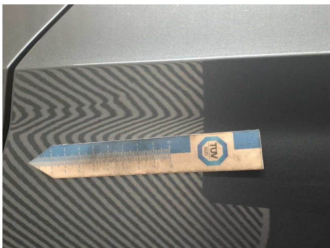
Damage 9: Door - rear left side: Door - dent(s) - Smart repair
