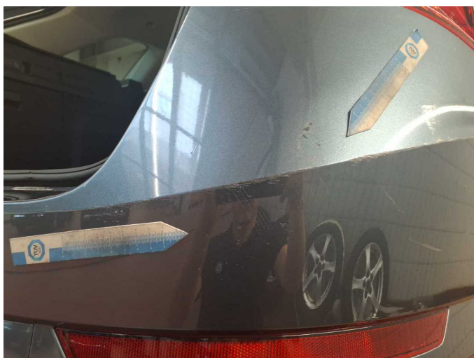
Damage 16: Rear bumper: Rear bumper - Scratched - Paint
