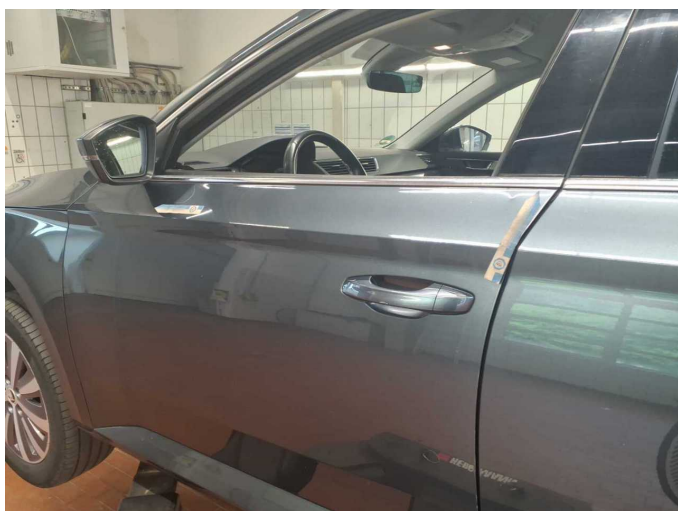
Damage 18: Door - front left side: Door (+ verschmutzt) - Dent / paintcoat damage - Repair and paint
