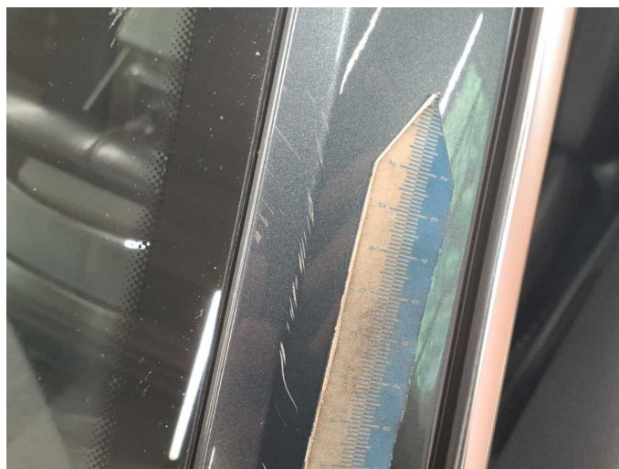
Damage 11: Body: A-pillar - left side - Scratch(es) - Smart repair
