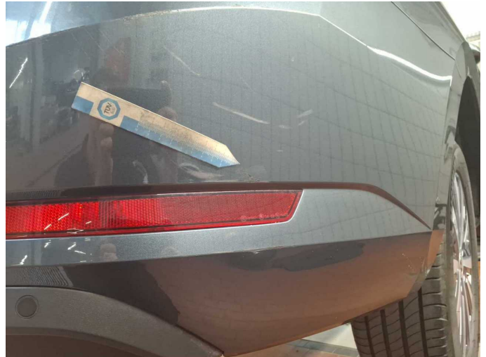
Damage 16: Rear bumper: Rear bumper - Scratched - Paint
