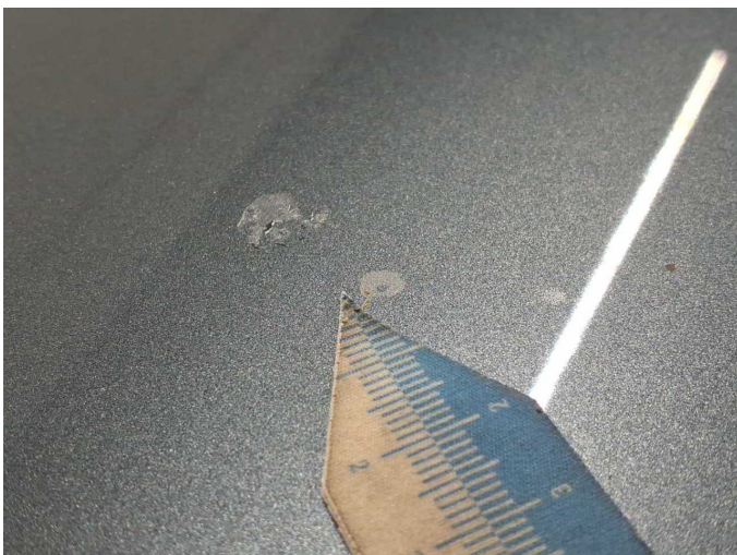
Damage 20: Bonnet: Bonnet (+ Steinschläge) - Paint defect - Paint
