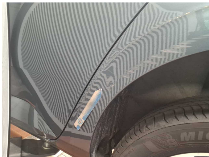
Damage 19: Side panel - rear left side: Side panel - Dent / paintcoat damage - Repair and paint
