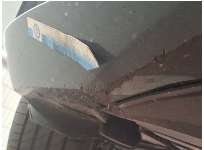
Damage 21: Front bumper: Front bumper (+ Fehlstellung) - Scratched - Repair and paint
