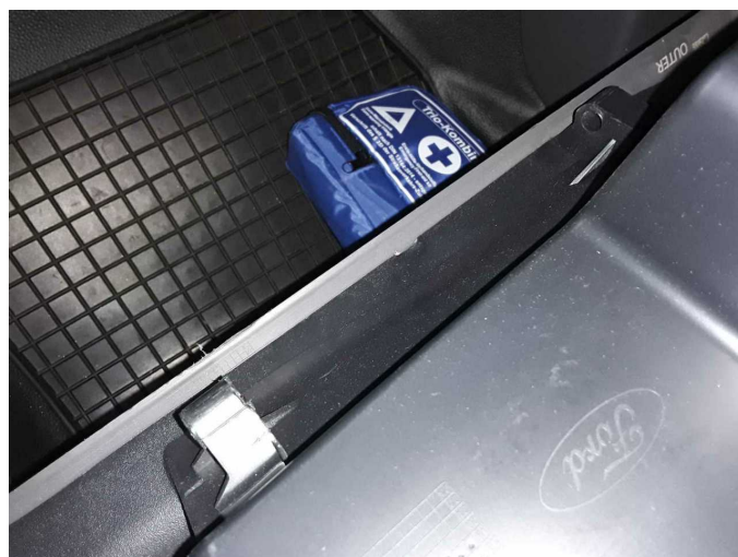
Damage 2: Instrument panel: Glove box - Loose - Repair
