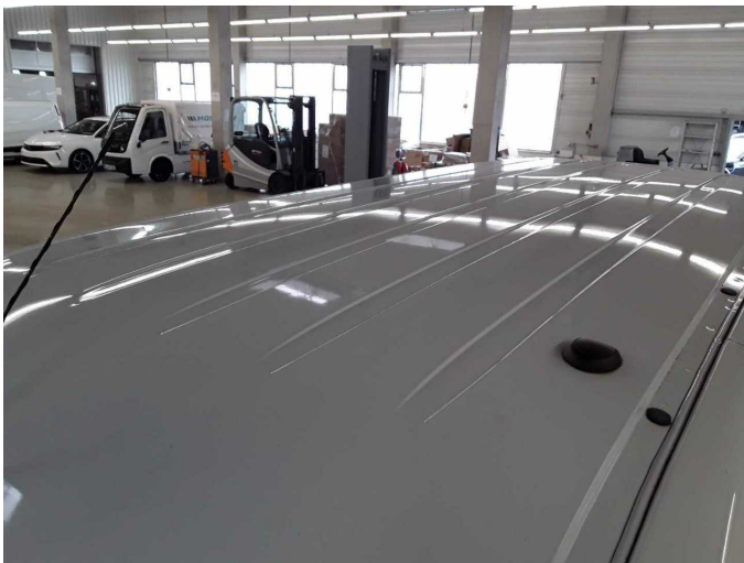
Damage 8: Roof: Roof - dent(s) - Smart repair
