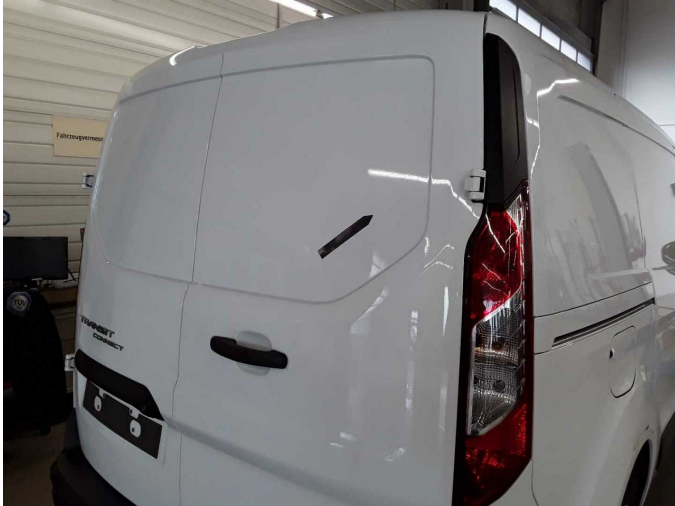
Damage 7: Boot lid / rear door: Rear door - right side - dent(s) - Smart repair
