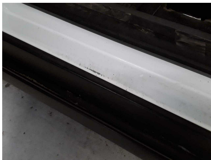
Damage 6: Sill - left side: Sill - Scratch(es) - Smart repair
