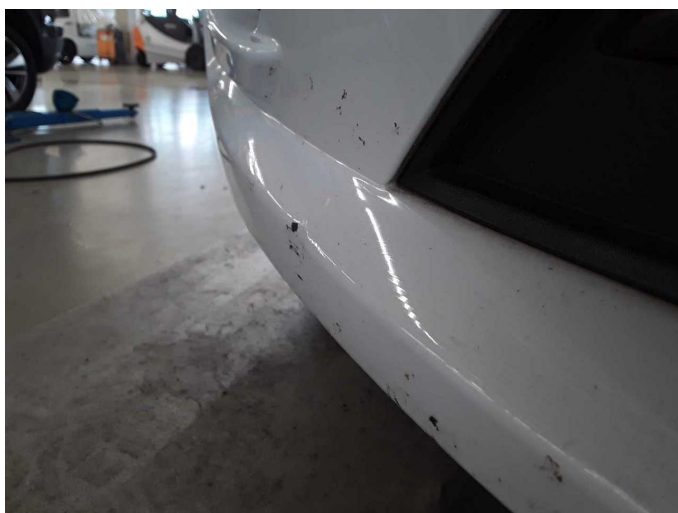
Damage 9: Front bumper: Bumper with Parktronic (Unterteil) - Deformed - Replace
