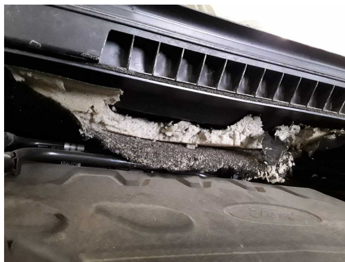
Damage 3: Cab: Insulation lining (Stirnband) - Damage caused by marten / rodent - Replace
