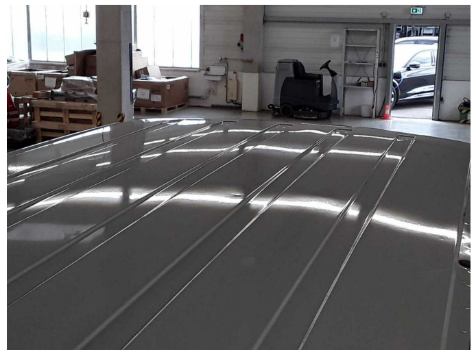
Damage 8: Roof: Roof - dent(s) - Smart repair
