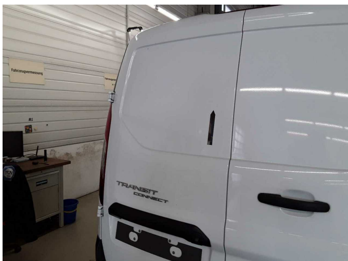
Damage 5: Boot lid / rear door: Rear door - left side - dent(s) - Smart repair
