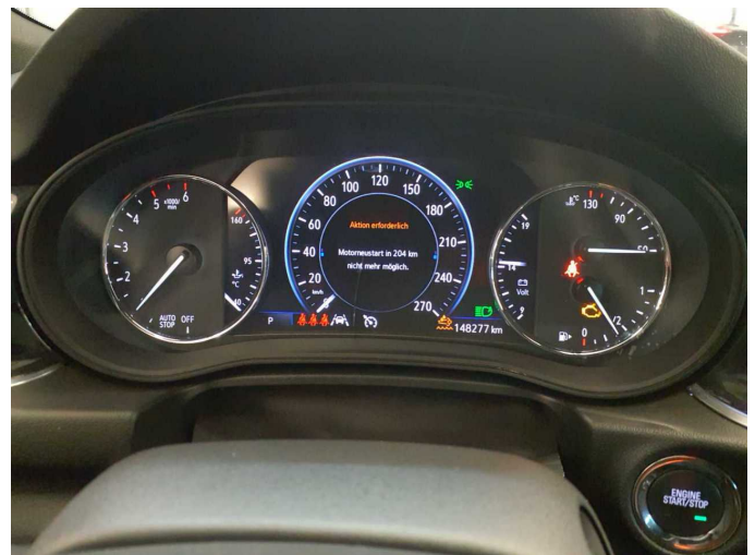
Wear and tear 2: Instrument panel: Indicator light (Ad Blue Nachfüllen!) - on - No deduction
