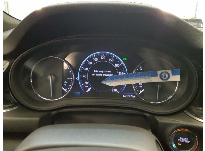
Damage 8: Instrument panel: Instrument cluster (Glas) - Broken / torn - Replace
