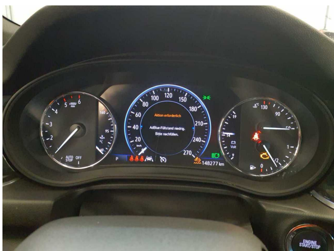
Damage 5: Instrument panel: Indicator light (Motorkontrollleuchte) - on - Perform diagnosis
