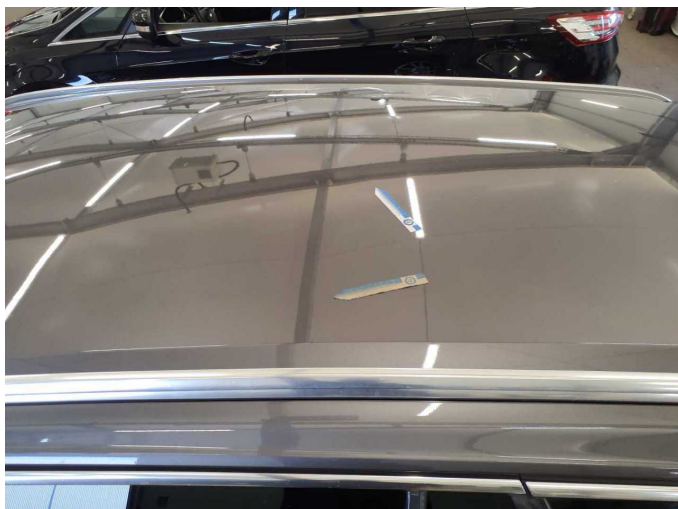
Damage 4: Roof: Roof - dent(s) - Smart repair
