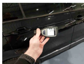
Paint thickness Door RR
