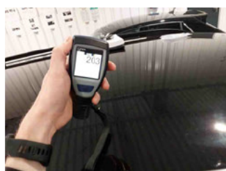
Paint thickness Roof
